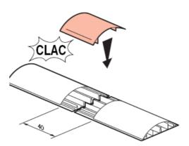
For mounting with floor ducts 92x20mm
