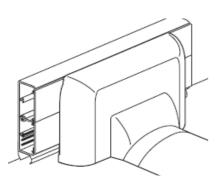
For branching from DLP trunking to floor duct Cat. No. 032800
