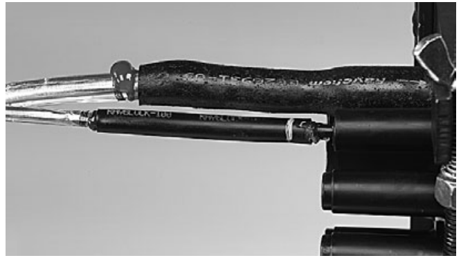
3.2.7 If cable is smaller than 5 mm, install built-up tubing 15 mm before the end of the outer jacket. Before installing, clean and abrade the cable.
