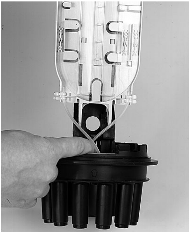
6.3 Cross-over for port 5 and 6, this for the top tray only.
