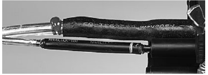
4.2.7 In case the cable has no strength member, push the built-up tubing 10 mm inside the round port. Clean and abrade the built-up tubing.
