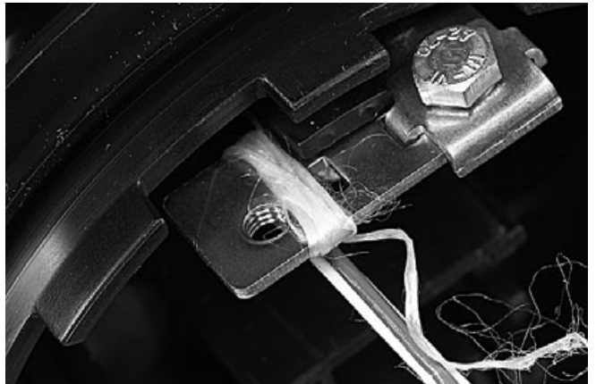
4.2.7 In case the cable has no strength member, push the built-up tubing 10 mm inside the round port. Clean and abrade the built-up tubing.
