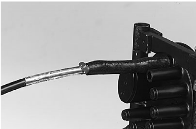
4.2.6 Hold the cable in position. Shrink till the green painting dots become black and the hotmelt is visible on the bottom. Do not move cable and closure until the adhesive is cooled down.
