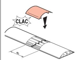
For mounting with floor ducts 92x20mm
