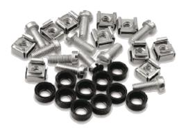
Inserting a panel into a rack becomes easy when a cage nut is used, the captive nut is clipped into the rack, then the screw is easily inserted as there is no need to hold the nut.
