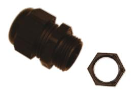
A cable gland offers good protection for incoming cables, suitable for different diameters ranging from 6mm to 14mm. As the gland is tightened is provides a seal around the cable.
