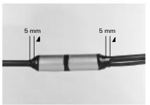
9 Tape maximum 5 mm onto the cable.
