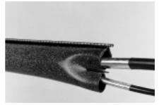
18 Insert the branch-off clip(s) completely between cables. Allow equal sleeve recovery space around cables.
