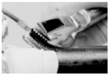
**4** Install shield continuity clip with standard pair of pliers.
