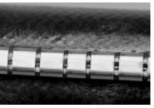
**24** When all temperature paint has been changed on the first half of the closure, two separate white lines should be visible in the slots of the channel.
