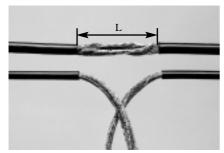
1 Remove cable jacket, following locally prescribed jointing techniques and hardware (length L). Maximum 3 cables at each end.
