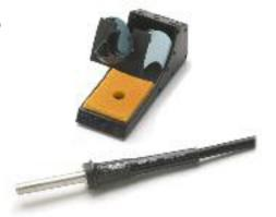
The HAP 200, 200 W/24 V, provides a directional hot airflow that is adjustable and static-free. Electronically temperature controlled from 50°C to 550°C. Different nozzles available as accessories. Finger switch controls speed adjustable pump. Hot air pencil set, consisting of HAP 200 with finger switch, WDH 30 Safety rest for pencil, nozzle 1,2 mm and 3,0 mm, key and nutdriver for nozzle changing.
