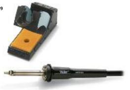
The HAP 1, 100 W/24 V, provides a directional hot airflow that is adjustable and static-free. Electronically temperature controlled from 50°C to 550°C. Different nozzles available as accessories. Finger switch controls speed adjustable pump. Hot air pencil set, consisting of HAP 1 with finger switch, WDH 30 Safety rest for pencil, nozzle 1,2 and 3,0 mm, key and nutdriver for nozzle changing.
