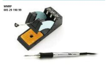
The RT soldering tips have an extremely short heat-up time. All component parts of the system, such as the sensor and heating element, are designed for optimum heat transfer. This ensures absolute efficiency in the utilization of the power provided by the supply unit. The recovery time is minimized. Changing soldering tips is quick, easy, and, most importantly, requires no tools. WMRP set, consisting of WMRP soldering pencil, RT 3 soldering tip and WDH 50 Safety rest.
