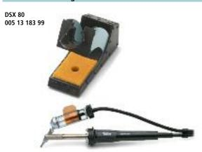
An 80 W/24 V desoldering iron for electronics rework. Electronically temperature controlled. Micro-finger switch controls quick-start, fast action vacuum pump. Different interchangeable tiplets, plus several CSF devices are available as accessories. DSX 80 set, consisting of DSX 80 Desoldering iron, WDH 30 Safety rest, cleaning tool, glass collector, two desoldering nozzles, gasbet, anti-bloc paste, filter.
