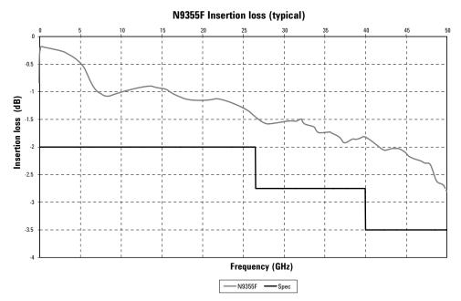
Figure 12. N9355F typical insertion loss versus frequency
