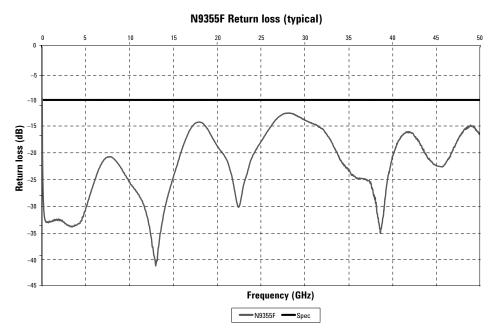
Figure 13. N9355F typical return loss versus frequency
