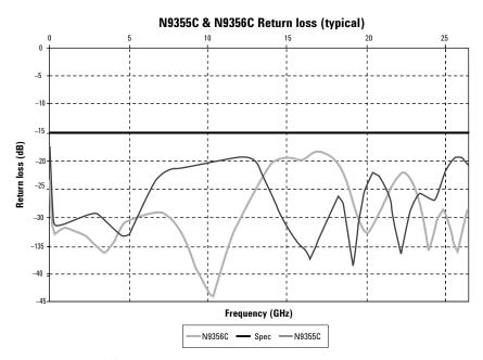
Figure 11. N9355/6C typical return loss versus frequency
