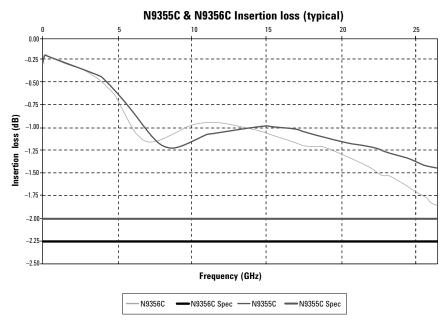
Figure 10. N9355/6C typical insertion loss versus frequency
