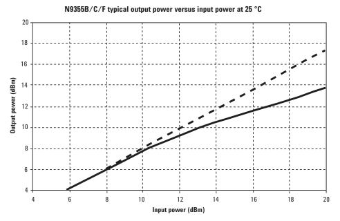
Figure 6. N9355B/C/F typical output versus input power
