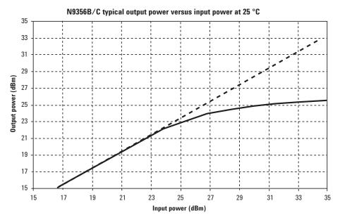
Figure 7. N9356B/C typical output versus input power
