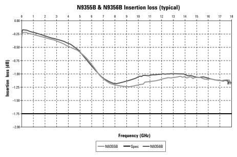
Figure 8. N9355/6B typical insertion loss versus frequency
