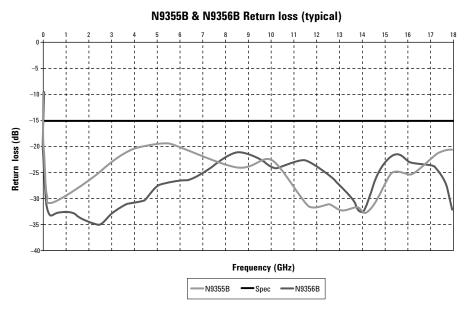
Figure 9. N9355/6B typical return loss versus frequency
