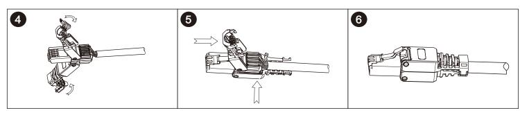
ACCORDING CABLE EXTERNAL DINAMETER, PUT PLASTIC WIRE GUARD INTO HOLDER HOLE LOKE THE ARROWHEAD
