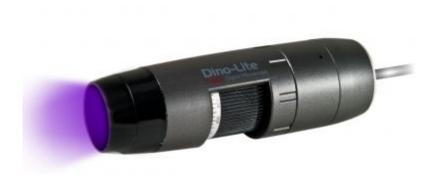
The Dino-Lite AM4115T-CFVW digital microscope is optimized for research and viewing fluorescent objects by using 400nm near UV excitation LEDs. It has a long-pass type 430nm emission filter that is designed to observe a wide range of fluorophores with applications in developmental biology, pathology, and anatomy.
