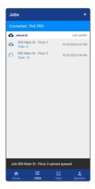
After the Job is uploaded, the arrow will change to a tick mark which indicates all tests in the Job are uploaded.
