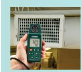
Convenient 4-in-1 Anemometer measures Air Velocity, Air Flow, Air Temperature, and Type K Temperature. Built-in low friction ball bearing mini vane wheel for high accuracy. The Type K temperature probe function measures surface temperature up to 2372°F (1300°). Features large dual LCD with backlighting, Data Hold, and Min/Max function.
