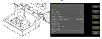
4. When pressure stick is withheld upwards, place the Short Bar in the central point of measuring electrode plate with recession facing upwards. Align the pressure stick with the Short Bar gently followed by pushing down the pressure stick into place so that the Short Bar, which contacts H/L 2-sides electrode plate, completes the short-circuit state. Execute the SHORT CORRECTION and the SHORT item will change from OFF to ON.
