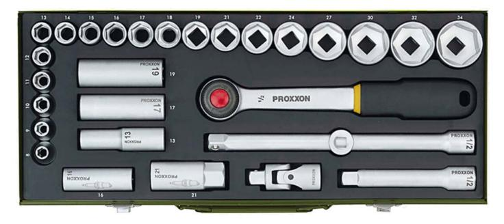
Sockets from 8 - 34mm (the latter for M 22 according to the new ISO standard). Deep sockets in sizes 13 - 17 and 19mm for protruding bolts. Spark plug sockets 16 and 21mm. See photo for full contents.
