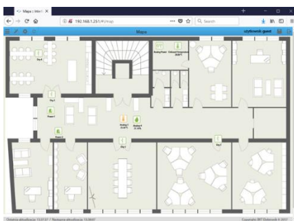
Visualization of sensor states on site layout from the device's web interface
